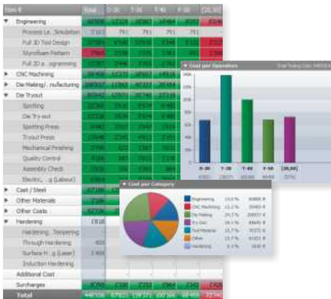
More consistent, more reliable and more rapid – AutoForm-CostEstimator provides tooling cost estimates based on 3D-CAD part data and stamping process
